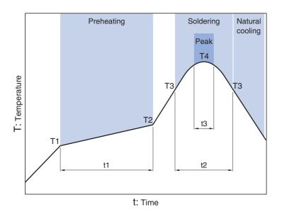
Preheating Soldering Peak Temp. Temp. Time Time Temp. Time **T1** T2 t1 ТЗ t2 Т4 t3 150°C 180°C 60 to 120s 230°C 260°C 30s 10s
