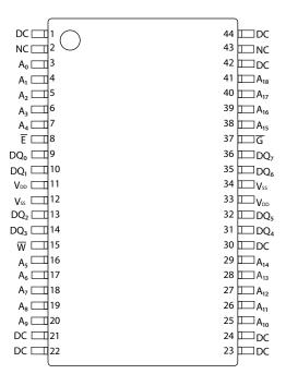
Figure 1.2 Pin Diagrams for Available Packages (Top View)
