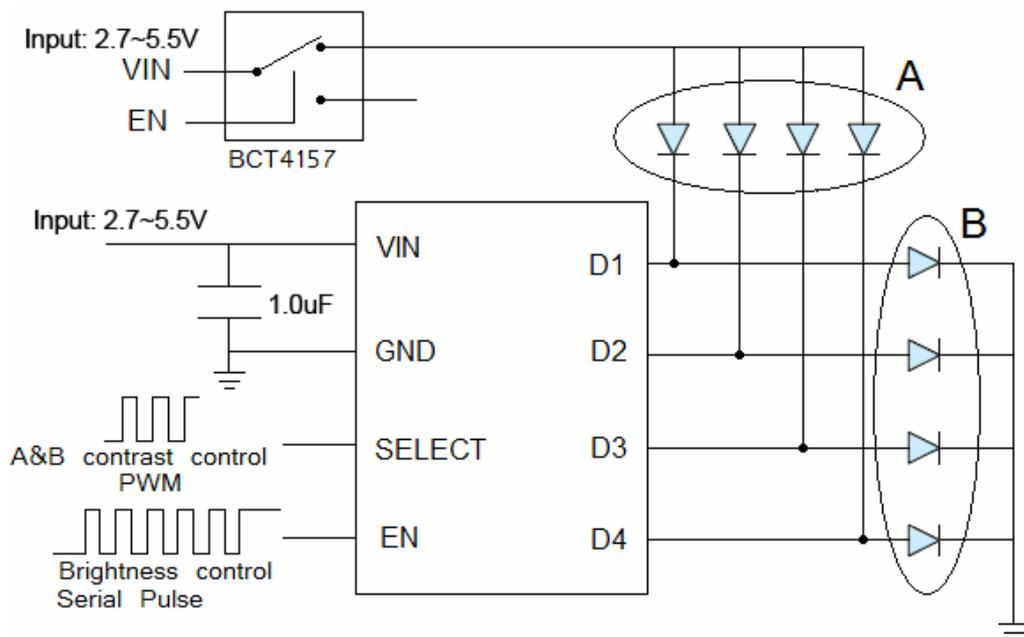
Figure 3: Application Circuit for Co-Anode & Co-Cathode Connection.
