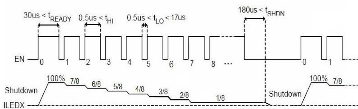
Figure 4: Brightness Control by Pulse Dimming
