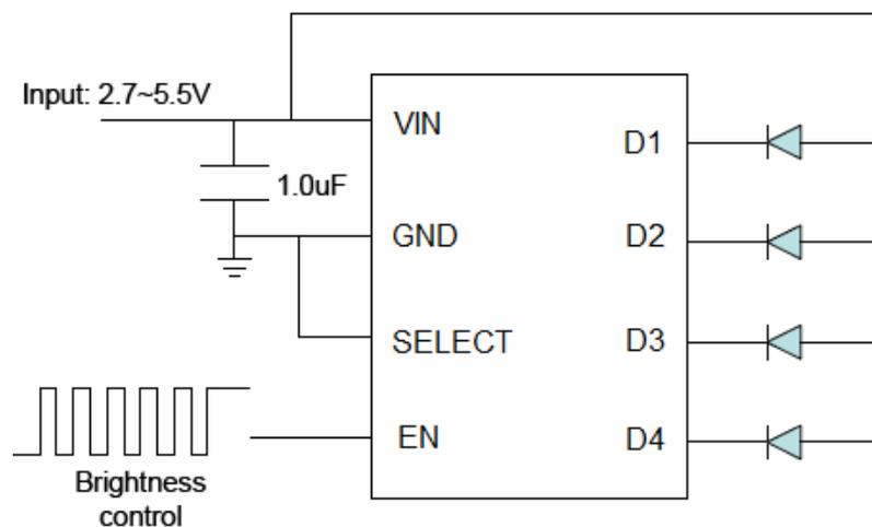
Figure 1: Application Circuit for Co-Anode Connection.
