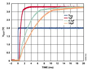
Figure 40.  $V_{OUT}$  Start-Up Time Behavior at Various Values of  $C_{BYP}$ ,  $V_{OUT} = 3.3~V$
