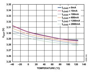
Figure 6. Output Voltage ( $V_{OUT}$ ) vs. Temperature at Various Loads,  $V_{OUT}$  = 3.3 V
