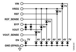
Figure 42. Simplified ESD Protection Block Diagram
