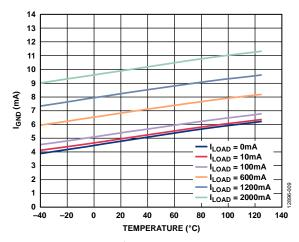
Figure 9. Ground Current ( $I_{GND}$ ) vs. Temperature at Various Loads,  $V_{OUT} = 3.3 \text{ V}$
