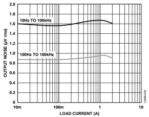
Figure 28. RMS Output Noise vs. Load Current
