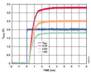
Figure 39.  $V_{OUT}$  Start-Up Time After  $V_{EN}$  Rising at Various Output Voltages,  $V_{IN} = 5 V$ ,  $C_{BYP} = 1 \mu F$
