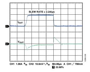
Figure 34. Load Transient Response,  $I_{LOAD} = 100$  mA to 2 A,  $V_{OUT} = 3.3$  V,  $V_{IN} = 4.0$  V,  $C_{OUT} = 22$   $\mu$ F, Channel 1 =  $I_{OUT}$ , Channel 2 =  $V_{OUT}$
