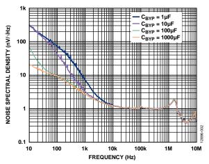
Figure 2. Noise Spectral Density at Various Values of  $C_{BYP}$ ,  $V_{OUT} = 3.3 \text{ V}$
