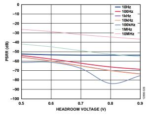
Figure 26. Power Supply Rejection Ratio (PSRR) vs. Headroom Voltage at Various Frequencies, V<sub>OUT</sub> = 1.8 V, 2 A Load
