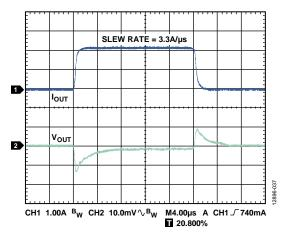
Figure 35. Load Transient Response,  $I_{LOAD} = 100$  mA to 2 A,  $V_{OUT} = 1.8$  V,  $V_{IN} = 2.5$  V, Channel  $1 = I_{OUT}$ , Channel  $2 = V_{OUT}$
