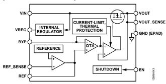
Figure 41. Simplified Internal Block Diagram
