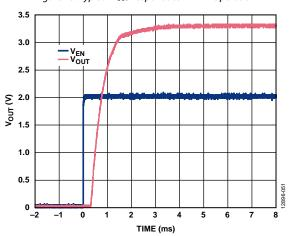
Figure 49. Typical  $V_{OUT}$  Response to EN Pin Operation ( $V_{EN}$ ),  $V_{OUT} = 3.3 \text{ V}$ ,  $V_{IN} = 5 \text{ V}$ ,  $C_{BYP} = 1 \mu F$
