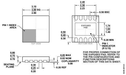
Figure 64. 10-Lead Lead Frame Chip Scale Package [LFCSP] 3 mm × 3 mm Body and 0.75 mm Package Height (CP-10-9) Dimensions shown in millimeters
