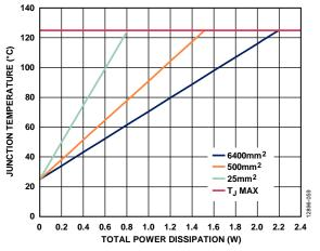
Figure 57. Junction Temperature vs. Total Power Dissipation for the 8-Lead SOIC,  $T_A = 25$ °C
