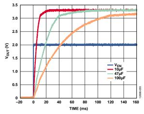
Figure 53. Typical Start-Up Behavior with  $C_{BYP} = 10 \, \mu F$  to  $100 \, \mu F$
