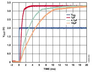
Figure 52. Typical Start-Up Behavior with  $C_{BYP} = 1 \mu F$  to  $10 \mu F$
