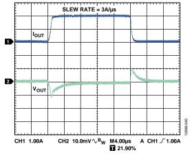
Figure 43. Output Transient Response,  $V_{OUT}$  = 3.3 V,  $C_{OUT}$  = 10  $\mu$ F, Channel 1 = Load Current, Channel 2 =  $V_{OUT}$
