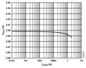
Figure 7. Output Voltage (Vout) vs. Load Current (ILOAD), Vout = 3.3 V
