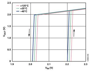
Figure 47. Typical UVLO Behavior at Various Temperatures,  $V_{OUT} = 3.3 \text{ V}$
