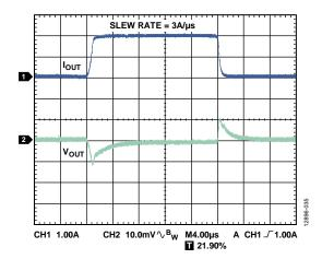
Figure 33. Load Transient Response,  $I_{LOAD} = 100$  mA to 2 A,  $V_{OUT} = 3.3$  V,  $V_{IN} = 4.0$  V, Channel  $1 = I_{OUT}$ , Channel  $2 = V_{OUT}$
