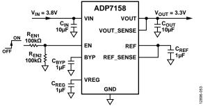
Figure 51. Typical EN Pin Voltage Divider
