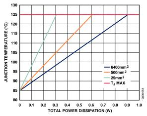
Figure 56. Junction Temperature vs. Total Power Dissipation for the 10-Lead LFCSP,  $T_A = 85^{\circ}C$
