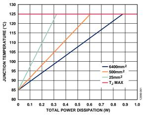
Figure 59. Junction Temperature vs. Total Power Dissipation for the 8-Lead SOIC,  $T_A = 85$ °C
