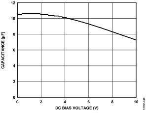
Figure 46. Capacitance vs. DC Bias Voltage
