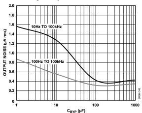
Figure 44. RMS Noise vs. Bypass Capacitance (CBYP)
