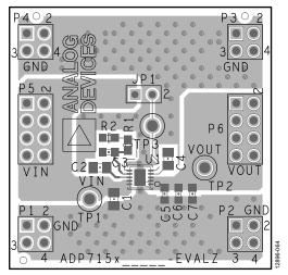
Figure 62. Sample 10-Lead LFCSP PCB Layout
