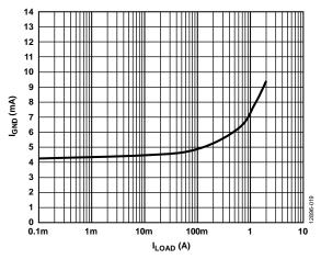
Figure 19. Ground Current (I<sub>GND</sub>) vs. Load Current (I<sub>LOAD</sub>), V<sub>OUT</sub> = 1.8 V
