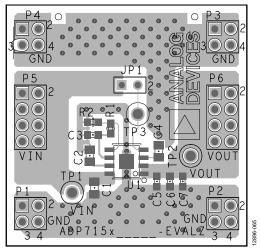
Figure 63. Sample 8-Lead SOIC PCB Layout
