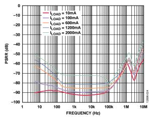
Figure 24. Power Supply Rejection Ratio (PSRR) vs. Frequency at Various Loads, V<sub>OUT</sub> = 1.8 V, V<sub>IN</sub> = 2.6 V
