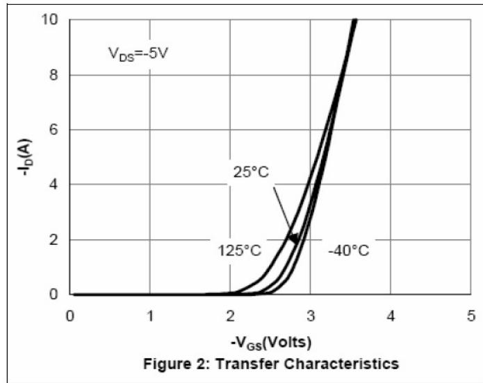
**Figure 2: Transfer Characteristics**
