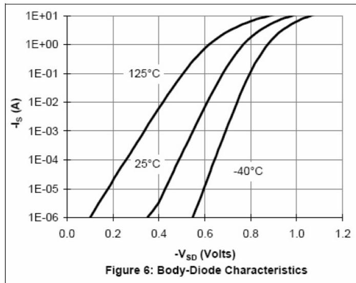
**Figure 6: Body-Diode Characteristics**
