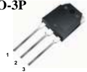
1.Gate 2. Drain 3. Source
