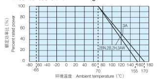
在环境温度70℃以上使用时,应按照上图负荷减轻特性曲线,减小额定功率。 For resistors operated at an ambient temperature of 70°C or above, a power rating shall be derated in accordance with the above derating curve.
