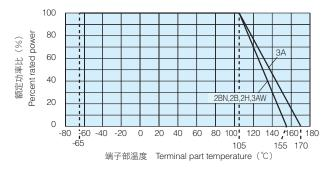
超过上述端子部温度使用时,请根据负荷减轻特性曲线减小额定功率后使用。 ※ 关于使用方法,请参照卷首的"端子部温度负荷减轻特性曲线的说明"。 For resistors operated terminal part temperature of described for each size or above, a power rating shall be derated in accordance with derating curve. \*\*Please refer to "Introduction of the derating curves based on the terminal part temperature" on the beginning of our catalog before use.
