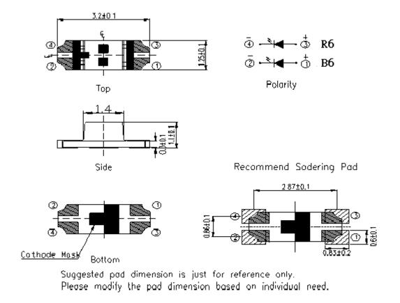
Note: Tolerances unless mentioned ±0.1mm. Unit = mm
