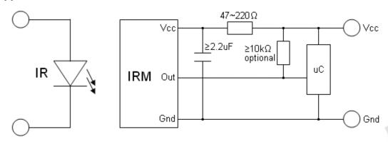
The RC Filter must be connected as close as possible to Vcc and GND pins.
