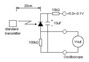
Fig.-3 Measuring System
