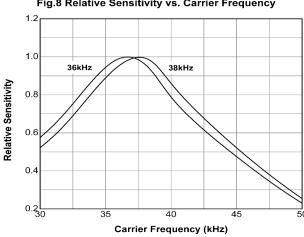
Fig.8 Relative Sensitivity vs. Carrier Frequency
