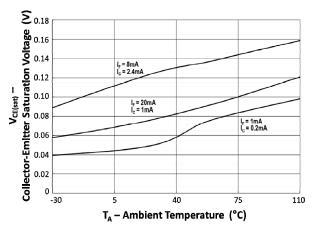
Fig 14 Collector-Emitter Saturation Voltage vs  $T_{\rm A}$
