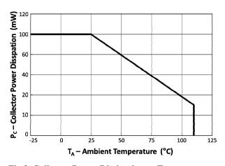
Fig 2 Collector Power Dissipation vs  $T_A$
