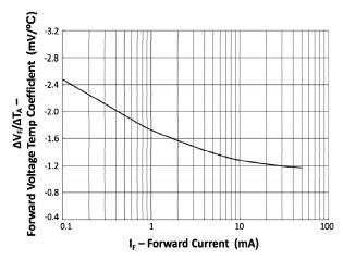
Fig 4 Forward Current Temperature Coefficient vs Forward Current
