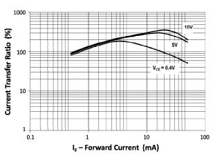
Fig 9 Current Transfer Ratio vs Forward Current
