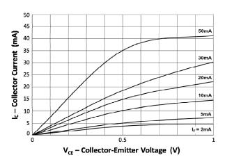
Fig 8 Collector Current vs Low Collector-Emitter Voltage
