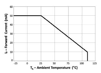
Fig 1 Forward Current vs T<sub>A</sub>
