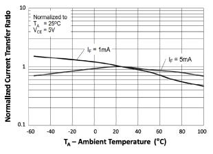
Fig 12 Normalized Current Transfer Ratio vs TA
