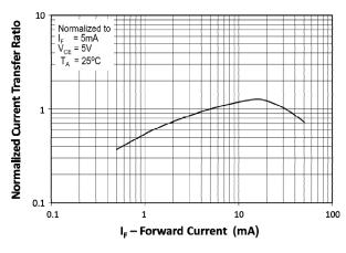
Fig 11 Normalized Current Transfer Ratio vs Forward Current
