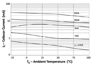
Fig 10 Collector Current vs T<sub>A</sub>
