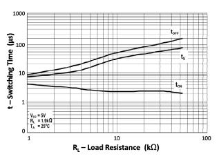
Fig 17 Switching Time vs Load Resistance
