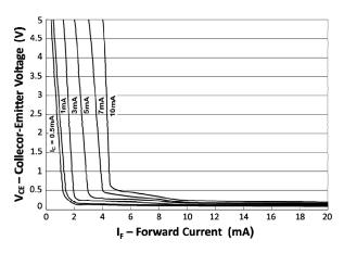
Fig 13 Collector-Emitter Voltage vs Forward Current
