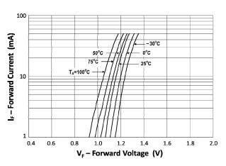
Fig 3 Forward Current vs Forward Voltage
