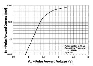
Fig 5 Pulse Forward Current vs Pulse Forward Voltage
