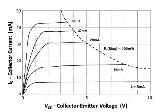
Fig 7 Collector Current vs Collector-Emitter Voltage
