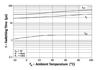
Fig 18 Switching Time vs  $T_A$
