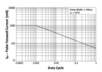
Fig 6 Pulse Forward Current vs Duty Cycle
