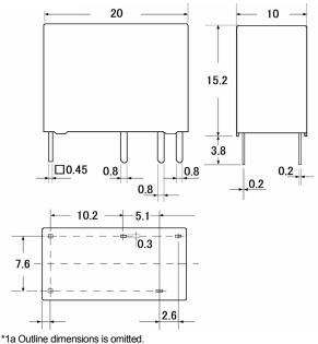
Tolerance: 0.99mm Max.: +/-0.1mm, 1-2.99mm: +/-0.2mm, 3mm Min.: +/-0.3r
