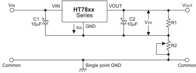
$$V_{OUT} = V_{xx} \left( 1 + \frac{R_2}{R_1} \right) + I_{SS} R_2$$
