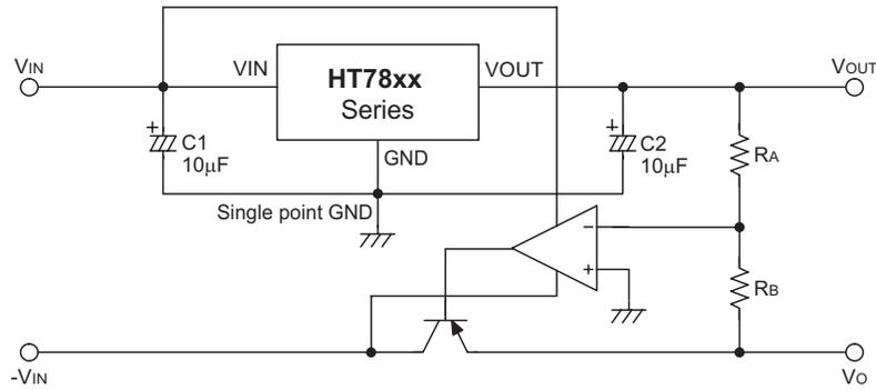
$$-V_o = V_{OUT} \times \frac{R_B}{R_A}$$
