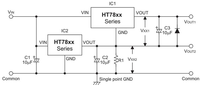
$$V_{OUT1} = V_{xx2} + V_{xx1}$$
