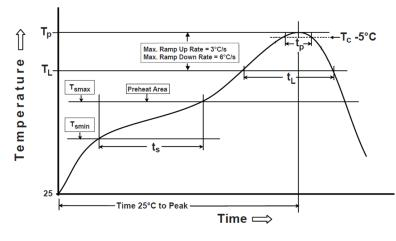
\* Recommended Temperature Profile for Wave Soldering
