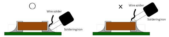
Fig 3 Correct handling method of soldering iron
