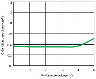
Fig 7. Capacitance vs. Reveres voltage
