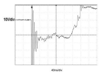
ESD clamping voltage Fig 9. (IEC61000-4-2-8KV contact)
