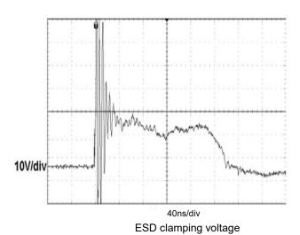
Fig 8. (IEC61000-4-2 +8KV contact)
