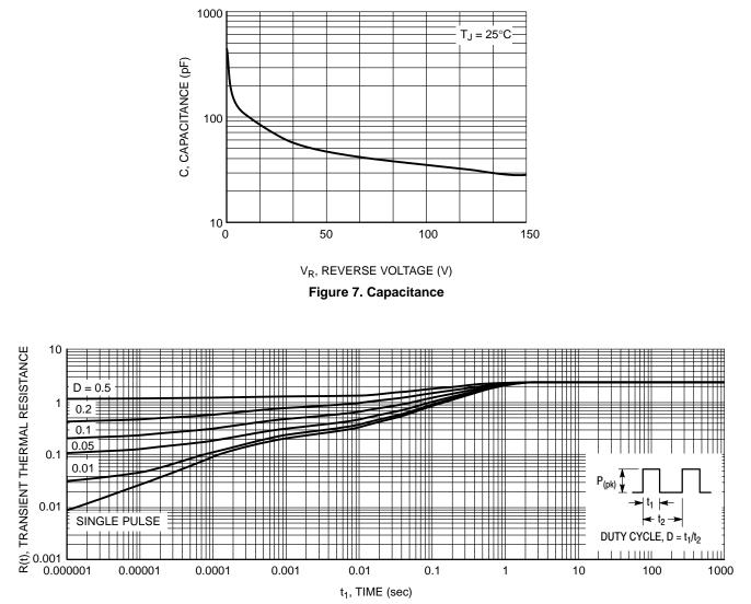
Figure 8. Thermal Response Junction-to-Case for MBRF10H150CTG
