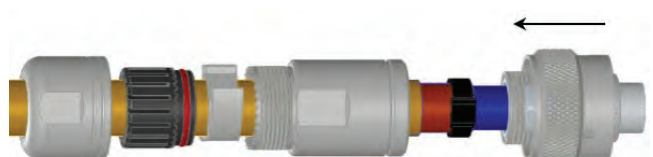
Step 6: Slide plug onto crimped terminal assembly
