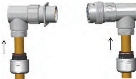
Step 11: Push shielding clip into backshell
