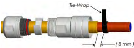
Step 3: Attach tie-wrap
