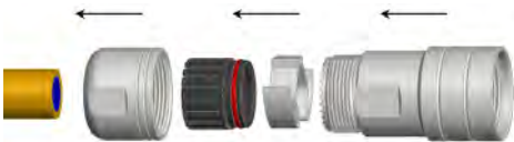
Step 1: Slide parts onto cable
