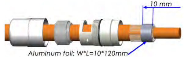
Step 4: Wrap foil over braided shielding
