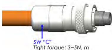
Step 9: Attach and tighten backshell as shown
