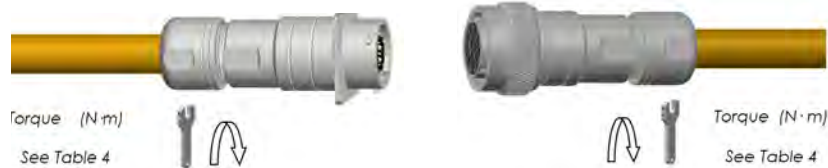
Step 13: Tighten metal nut
