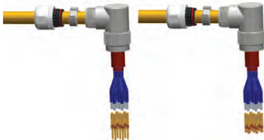
Step 7: Attach contacts to wire leads
