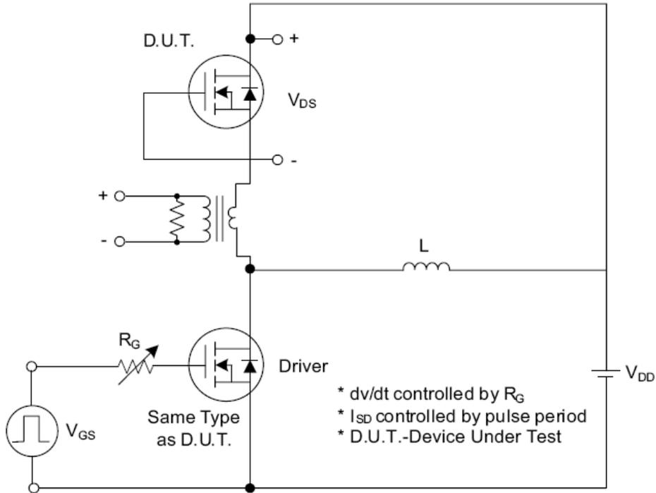
Fig. 1.1 Peak Diode Recovery  $dv/dt$  Test Circuit
