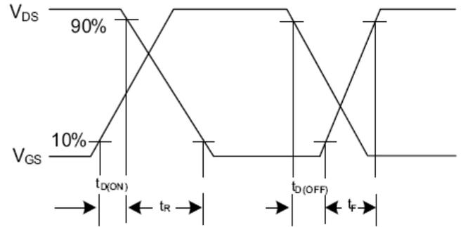
Fig. 2.2 Switching Waveforms
