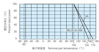
超过上述端子部温度使用时,请根据负荷减轻特性曲线减小额定功率后使用。 ※ 关于使用方法,请参照卷首的"端子部温度负荷减轻特性曲线的说明"。 For resistors operated terminal part temperature of described for each size or above, a power rating shall be derated in accordance with derating curve. \*\*Please refer to "Introduction of the derating curves based on the terminal part
