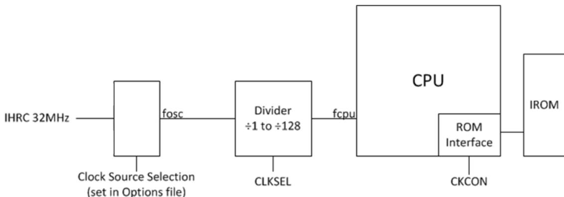
ROM interface is built in between CPU and IROM (program memory). It optionally extends the data fetching cycle in order to support lower speed program memory. For example if the CPU is anticipated to run at 32 MHz and the IROM has to run at 8 MHz, three extended cycle must be placed by CKCON register.
