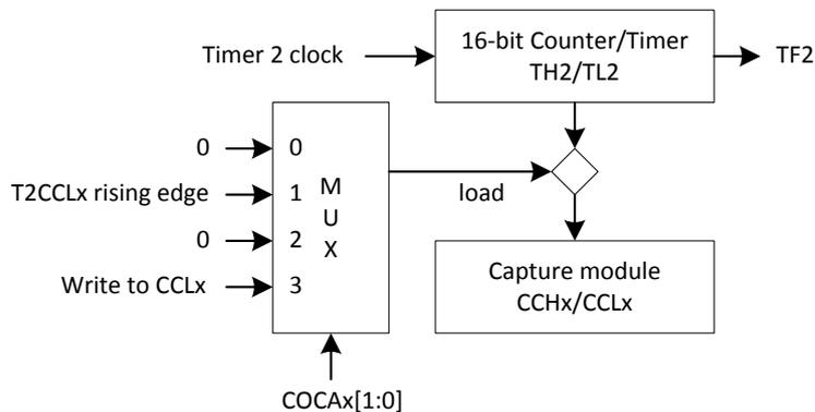
The split event can from hardware or software. The T2CC0 pin can trigger a hardware split event that duplicates TH2/TL2 value to CRCH/CRCL registers, whereas T2CC1, T2CC2 and T2CC3 respectively control CC1 to CC3 registers.
