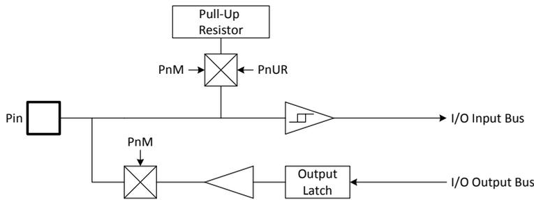
Bi-direction I/O Pin Shared with Specific Digital Input Function, e.g. INT0, Event counter, SIO, UART.
