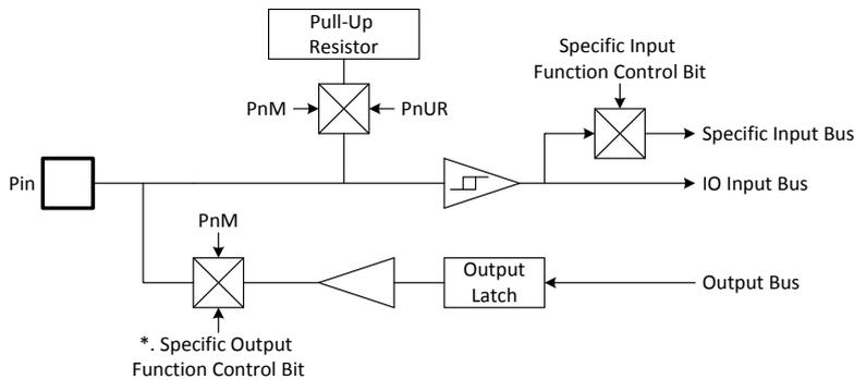
\*. Some specific functions switch I/O direction directly, not through PnM register.
