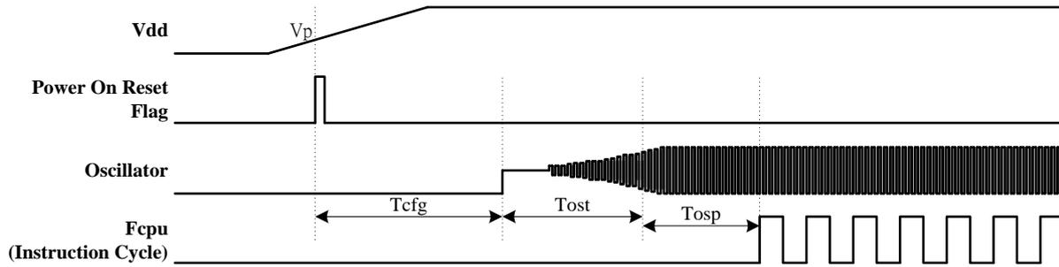
● External Reset Pin Reset Timing
