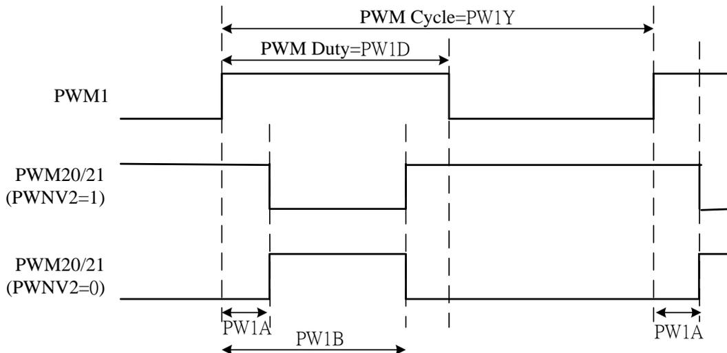
The PWM dead band occurs in PWM high pulse width, and the dead band period is programmable from  $PW1A$  and  $PW1D-PW1B$  registers. The dead band period is symmetrical at left-right terminal of PWM pulse width or not. If the dead band period is longer than PWM duty, the PWM is no output.
