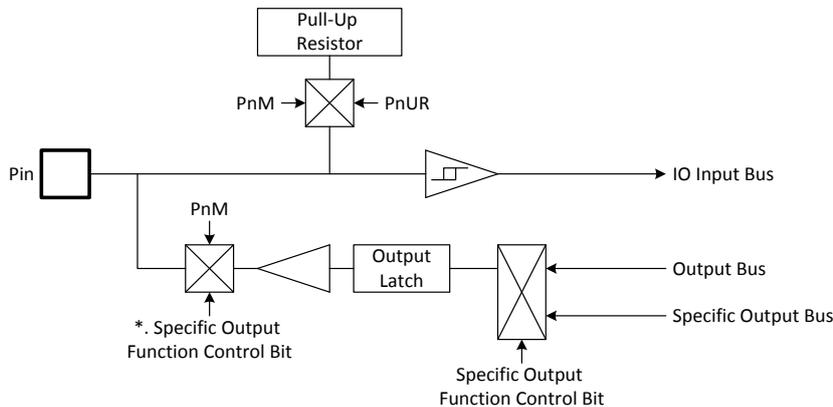
\*. Some specific functions switch I/O direction directly, not through PnM register.
