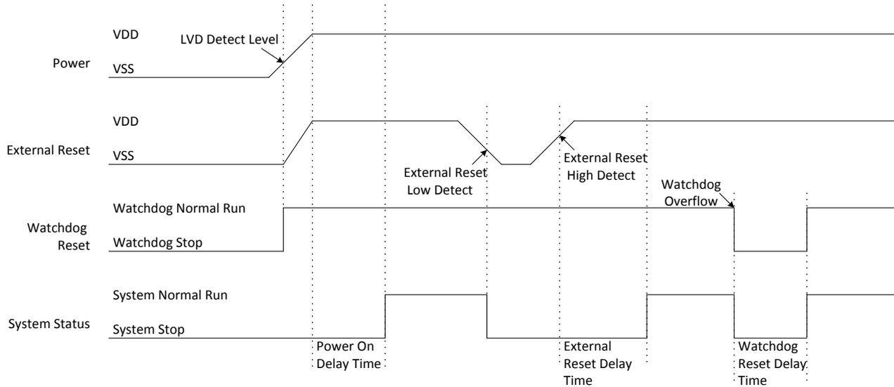
The power stabilization period spends 5 ms in typical condition. Afterward the microcontroller fetches CPU Clock Source selection automatically. The selected clock source would be driven, and the system counts 4096 times of the clock period to ensure its reliability.
