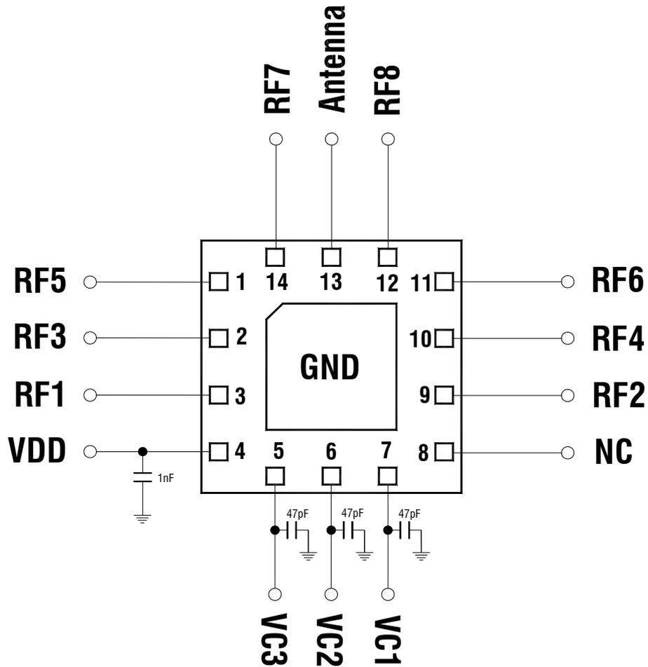
1. RF input and output are 50-Ohm microstrip.
