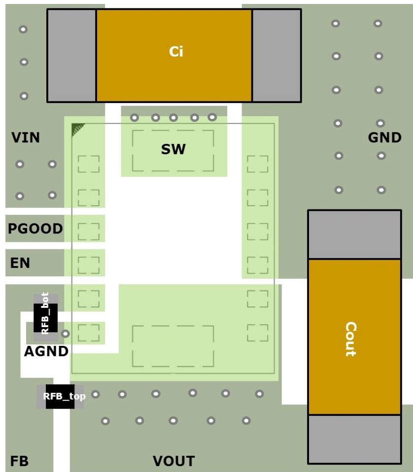
FIG.34 RECOMMENDATION LAYOUT (TOP LAYER)
