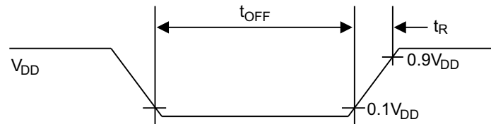
Figure 124. Low Voltage Reset Timing
