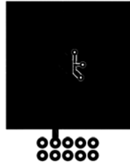
b. 50^\circ\text{C/W} when mounted on a 1\text{ in}^2 pad of 2 oz copper
