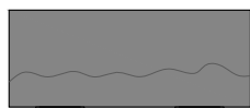
Severely crack: not acceptable. More obvious cracks extended from side to side.
