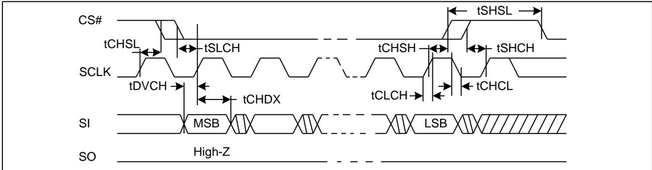
**Figure22. Output Timing**
