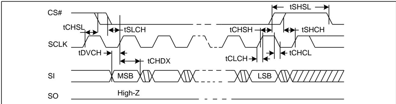
**Figure22. Output Timing**
