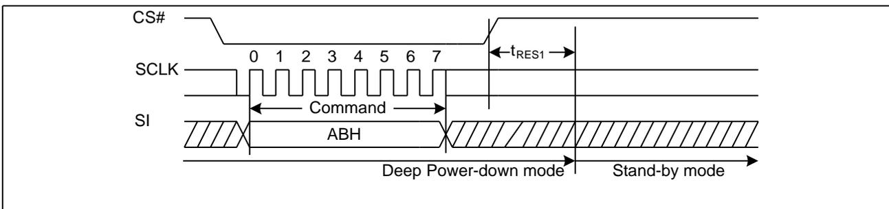
Figure15. Release Power-Down and Read Device ID Sequence Diagram
