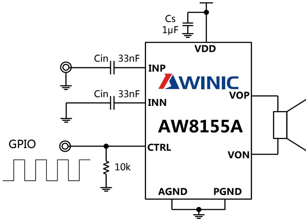
Figure 2. AW8155A Application Schematic With Single-Ended Input
