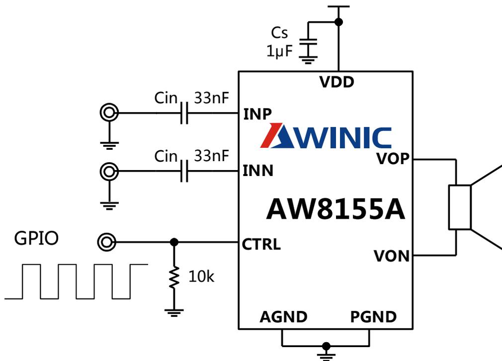
Figure 3. AW8155A Application Schematic With Differential Input
