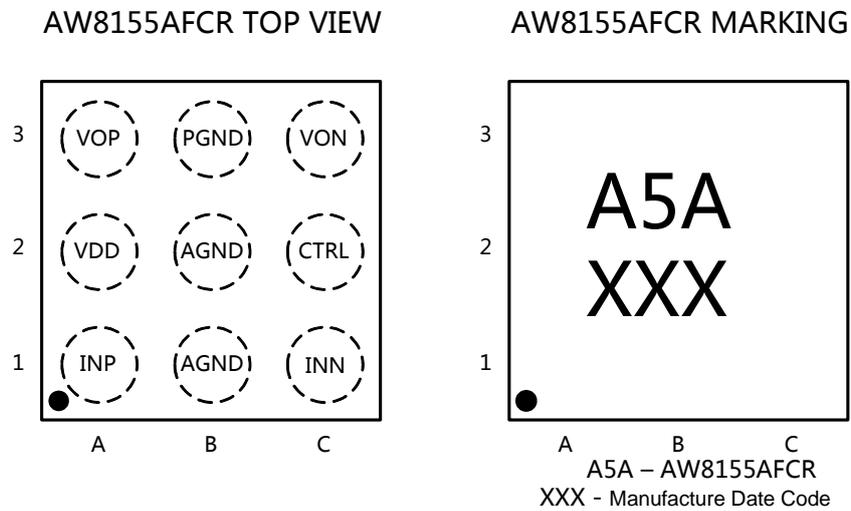
Figure 1. Pin Configuration and Top Mark of AW8155A
