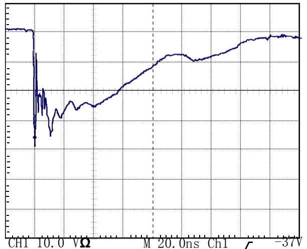
Figure 3 ESD Clamping Voltage Screenshot Negative 8 kV contact per IEC 61000-4-2
