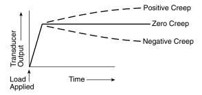
Since transducer creep depends on several variables such as spring element material, heat treatment, strain field, adhesive type and test temperature, it is not possible to predict the proper gage compensation necessary to achieve the best creep result.
