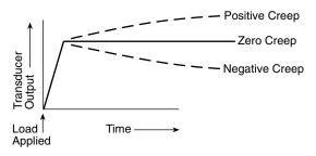
Since transducer creep depends on several variables such as spring element material, heat treatment, strain field, adhesive type and test temperature, it is not possible to predict the proper gage compensation necessary to achieve the best creep result.
