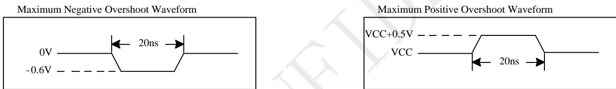
Figure 5-1 Maximum Overshoot Waveform
