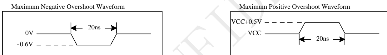
Figure 5-1 Maximum Overshoot Waveform
