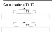
Each terminal extends the full of the **DPX162690DT-8039B1**. Hence any coplanarity deviation between terminals is due to curvature in the substrate. TDK guarantees that the edge of each terminal is within 0.05mm of the horizontal plane.
