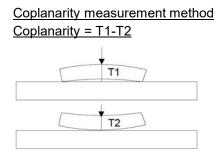
Each terminal extends the full of the product. Hence any coplanarity deviation between terminals is due to curvature in the substrate. TDK guarantees that the edge of each terminal is within 0.05 mm of the horizontal plane.
