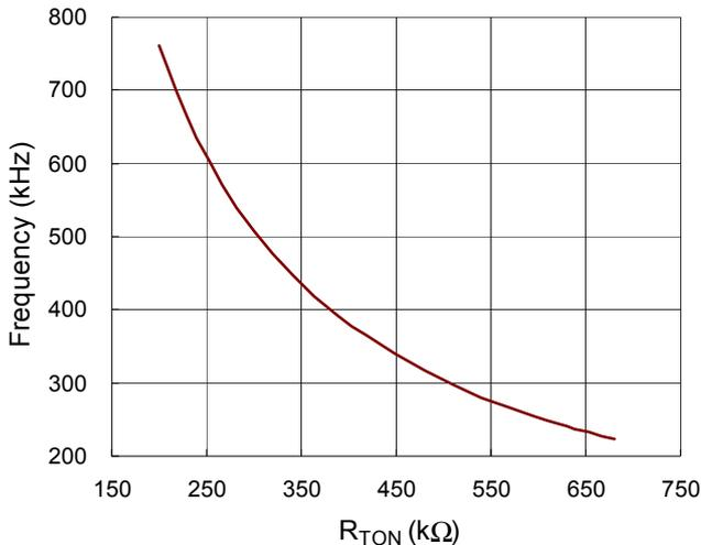
Figure 6. Frequency vs. R<sub>TON</sub>
