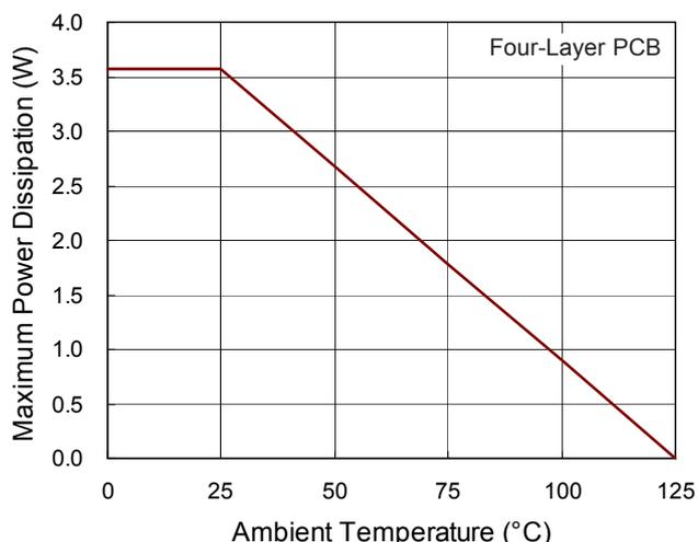
Figure 14. Derating Curve of Maximum Power Dissipation
