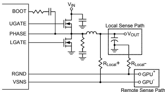
Figure 4. Output Voltage Sensing
