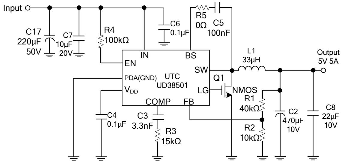
$$V_{OUT} = V_{FB} \times (1 + R1/R2), \quad V_{FB} = 1.00V, \quad R2 \text{ suggest } 10k \sim 30k\Omega$$
