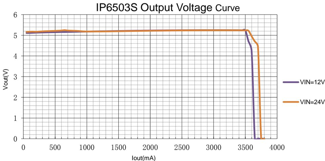
Fig.4 IP6503S Output Voltage Characteristics
