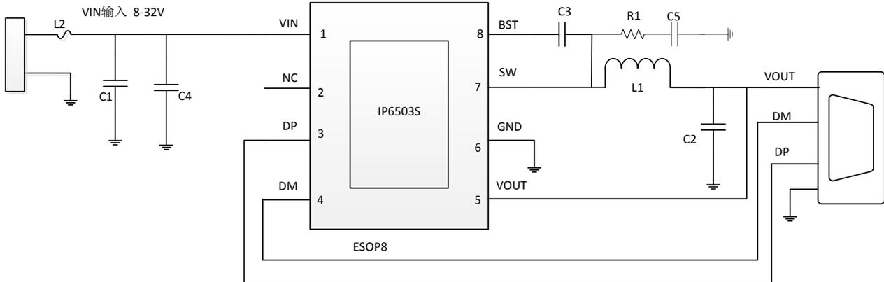
Fig. 1 IP6503S Simplified Schematic
