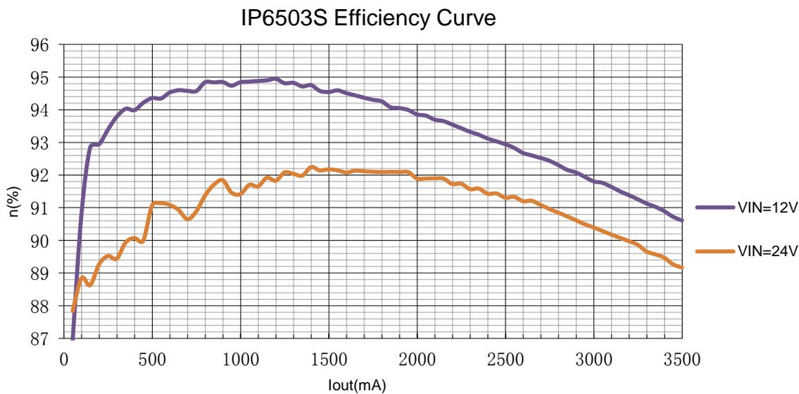
Fig. 3 IP6503S Conversion Efficiency
