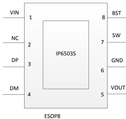
Fig. 2 IP6503S PIN Configuration
