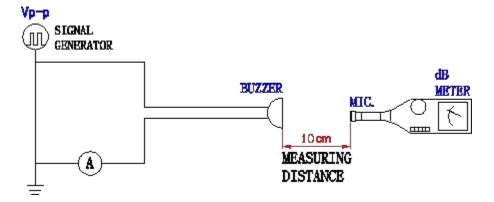
In the measuring test, buzzer is placed as follows:
