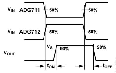
Figure 14. Switching Times
