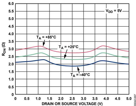
Figure 5. On Resistance as a Function of  $V_D$  ( $V_S$ ) for Different Temperatures
