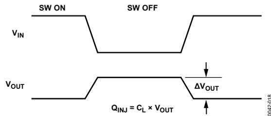
Figure 16. Charge Injection
