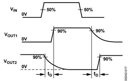
Figure 15. Break-Before-Make Time Delay,  $t_D$
