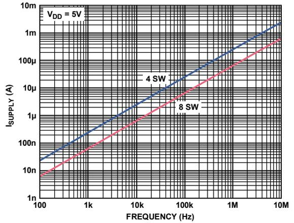
Figure 6. Supply Current vs. Input Switching Frequency
