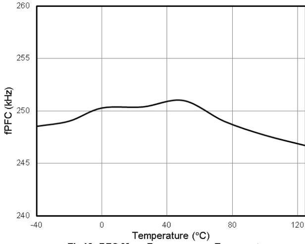
Fig13. PFC Max. Frequency vs. Temperature
