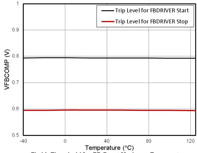
Fig14. Threshold for FB Burst Mode vs. Temperature
