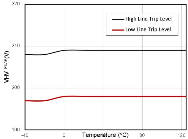
Fig2. High/Low Line Detection Trip Level vs. Temperature
