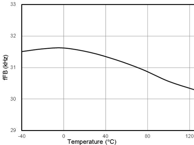
Fig5. QR Flyback Green Mode Frequency vs. Temperature
