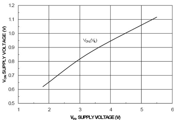
Figure 9.  $V_{ON}$  Low Voltage vs. Input Voltage
