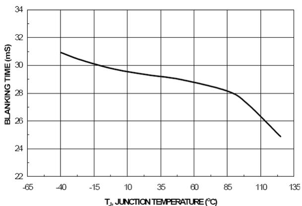
Figure 17. t<sub>BLANK</sub> vs. Temperature
