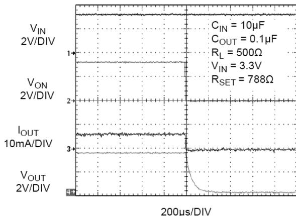
Figure 19. t<sub>OFF</sub> Response
