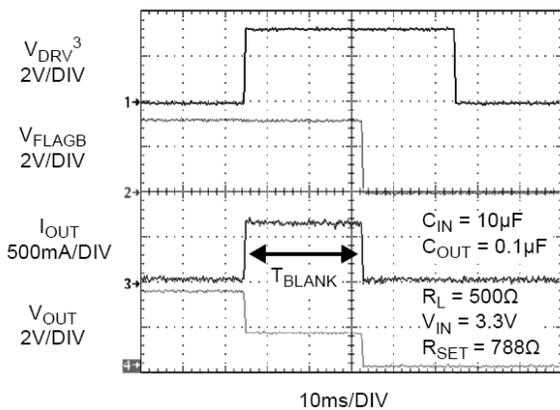
Figure 25.  $t_{BLANK}$  vs. Response<sup>(3)</sup>
