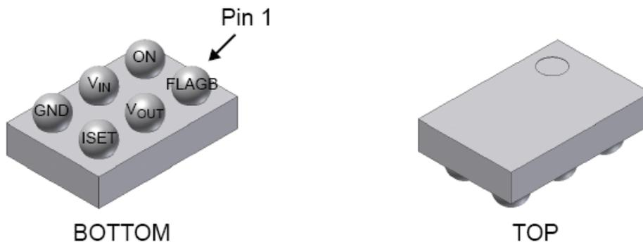
Figure 3. 1.0 x 1.5 mm Chip-Scale Package
