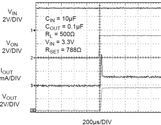
Figure 18. t<sub>ON</sub> Response
