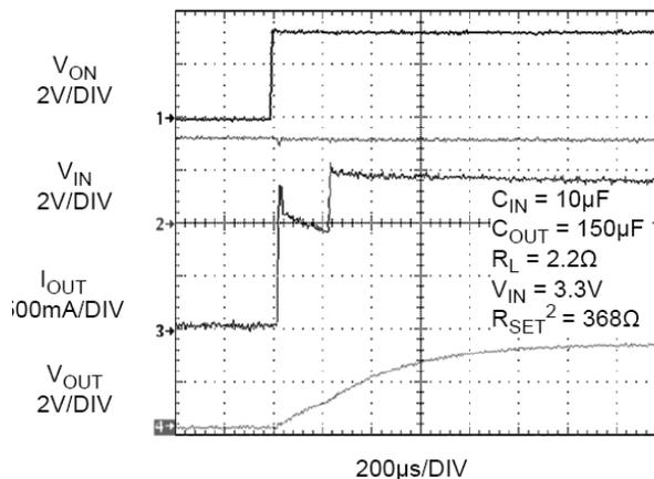
Figure 24. Short-Circuit Detection Function<sup>(4)</sup>
