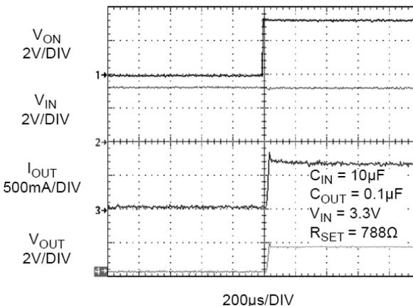
Figure 22. Current Limit Response Time (Output is Loaded by 2.2 Ω, C<sub>OUT</sub>=0.1 µF)
