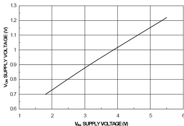
Figure 8.  $V_{ON}$  High Voltage vs. Input Voltage
