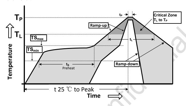
Figure 9 Recommended Lead-Free Reflow Profile
