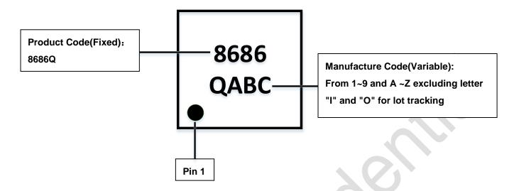
Figure 7 Marking specification (Top View)
