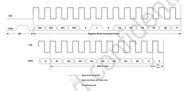
Figure 3 Register Write Command Sequence
