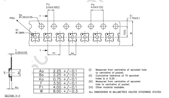
Figure 8 Tape and reel dimensions
