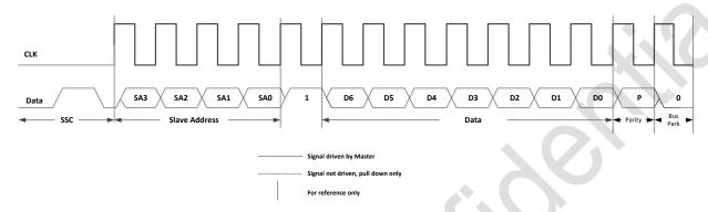
Figure 5 Register 0 Write Command Sequence
