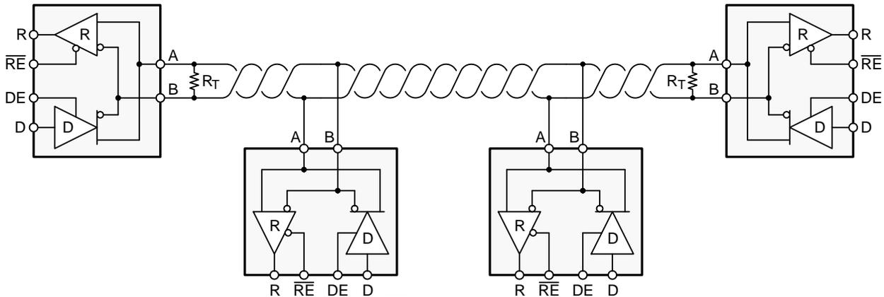
**Figure 20. Typical RS-485 Network With 65HVD7x Transceivers**
