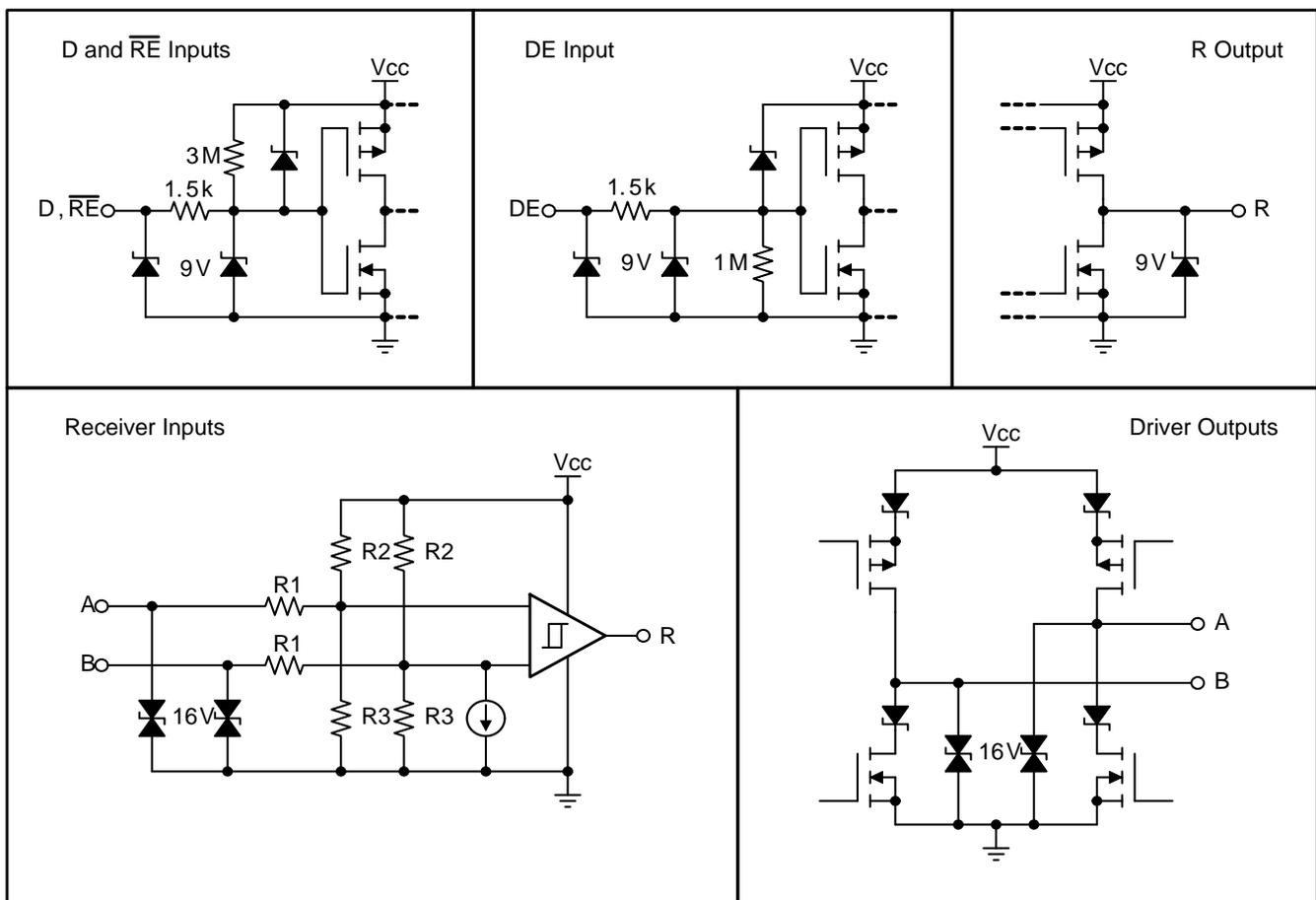
**Figure 18. Equivalent Input and Output Circuit Diagrams**
