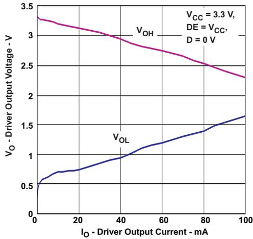
**Figure 1. Driver Output Voltage vs Driver Output Current**
