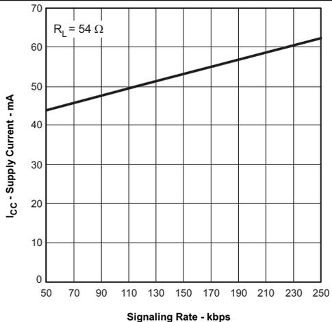
**Figure 6. 65HVD72 Supply Current vs Signal Rate**
