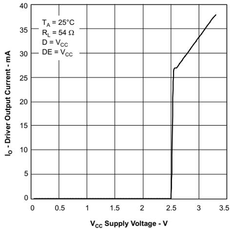
**Figure 3. Driver Output Current vs Supply Voltage**
