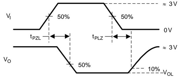
D at 0 V to test non-inverting output, D at 3 V to test inverting output.
