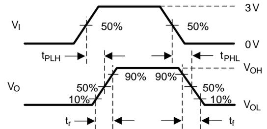
Figure 15. Measurement of Receiver Output Rise and Fall Times and Propagation Delays
