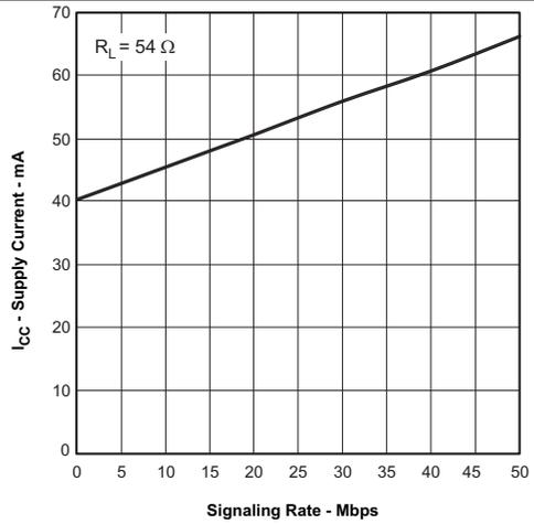
**Figure 8. 65HVD78 Supply Current vs Signal Rate**
