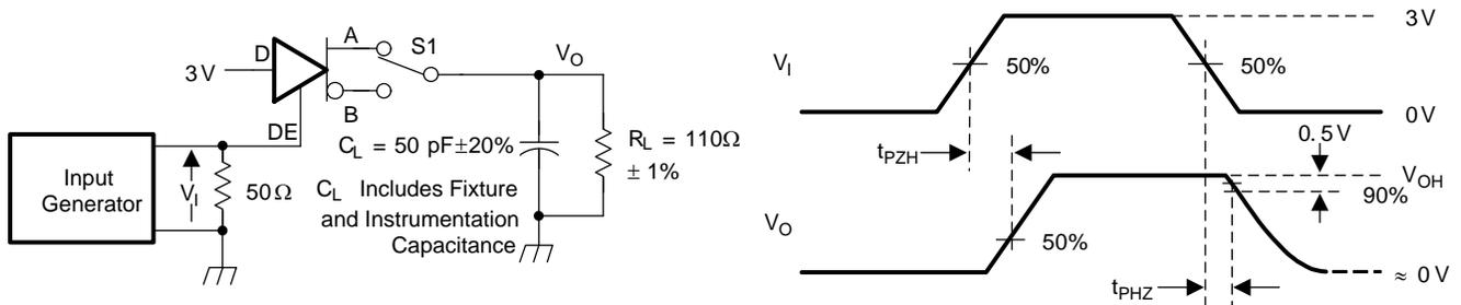
D at 3 V to test non-inverting output, D at 0 V to test inverting output.
