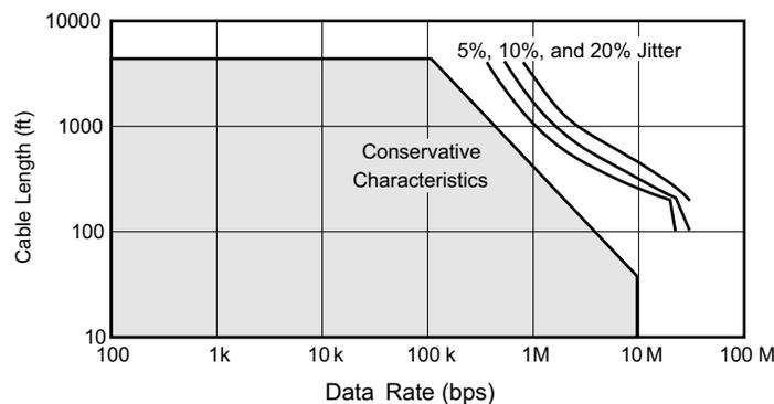
**Figure 21. Cable Length vs Data Rate Characteristic**
