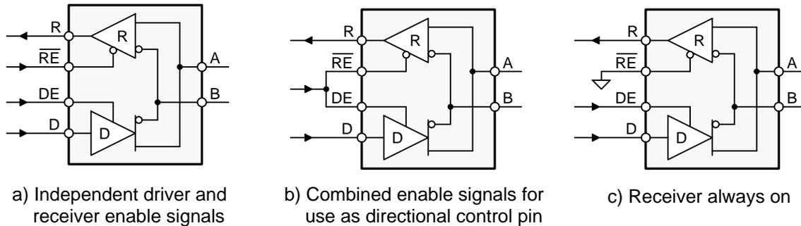
**Figure 19. Transceiver Configurations**
