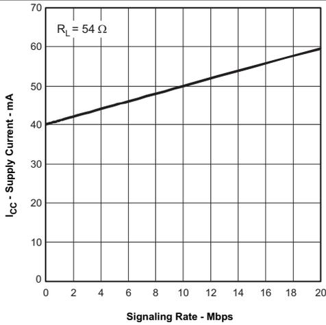
**Figure 7. 65HVD75 Supply Current vs Signal Rate**
