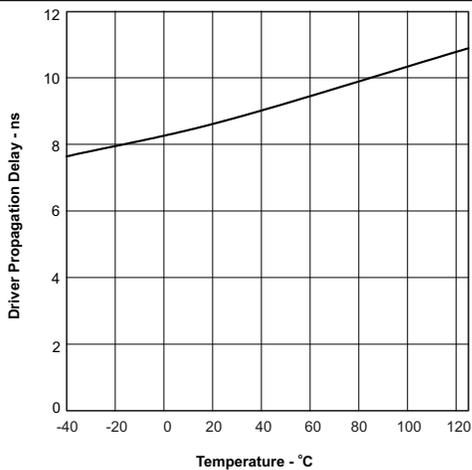
**Figure 5. 65HVD78 Driver Propagation Delay vs Temperature**
