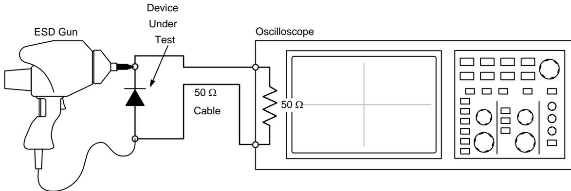
Figure 8. Diagram of ESD Clamping Voltage Test Setup
