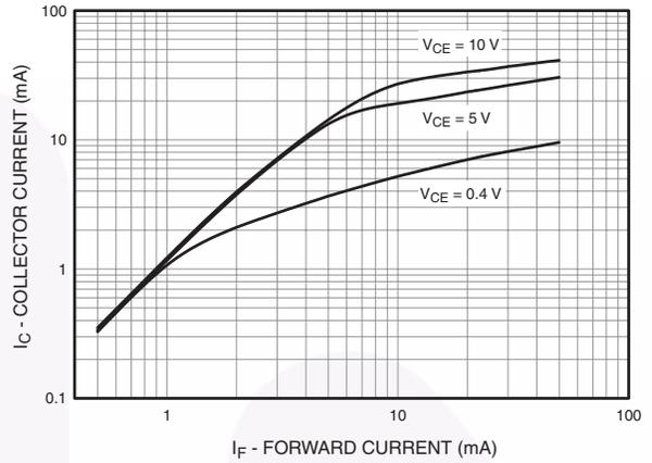
Fig. 3 Current Transfer Ratio vs. Forward Current
