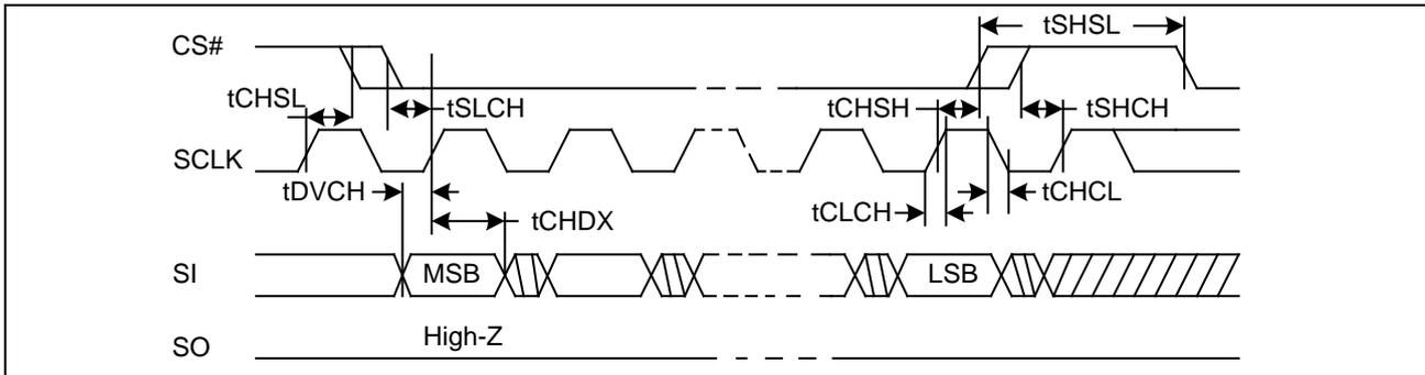
**Figure23. Output Timing**
