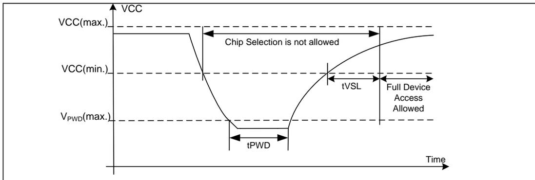
Table 5. Power-Up Timing and Write Inhibit Threshold
