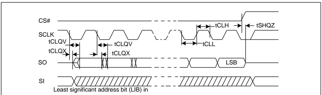
Figure 43. Resume to Suspend Timing Diagram
