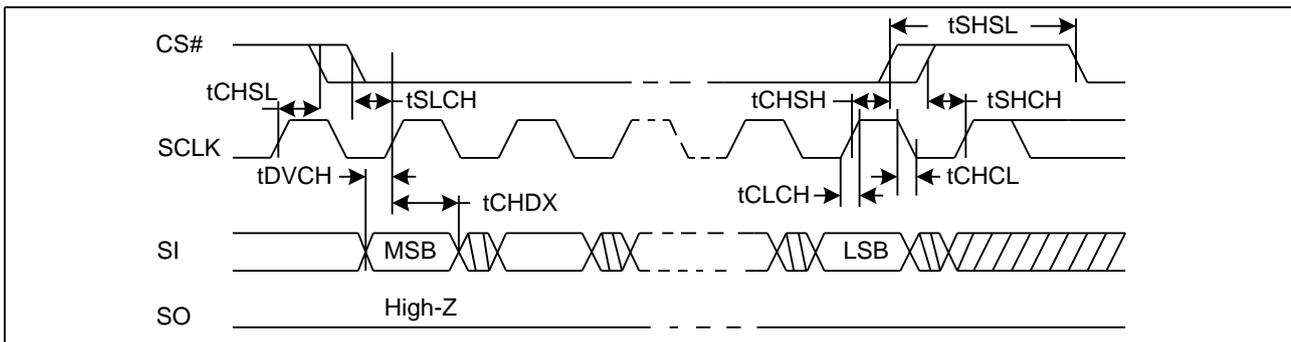
**Figure 42. Output Timing**
