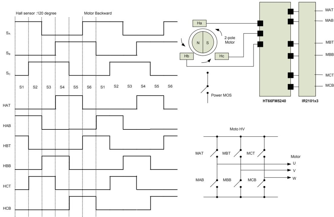
**Motor Drive Signal Timing Diagram – Backward Direction**
