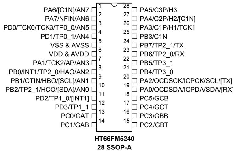
Note: The “VDD&AVDD” means that the VDD and AVDD are internally bonded while the “VSS&AVSS” means that the VSS and AVSS are internally bonded.
