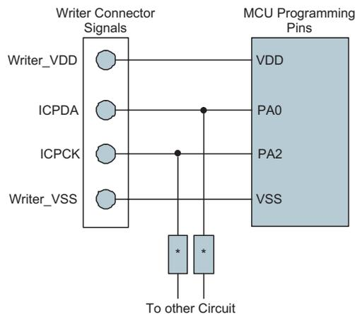
Note: \* may be resistor or capacitor. The resistance of \* must be greater than 1k or the capacitance of \* must be less than 1nF.
