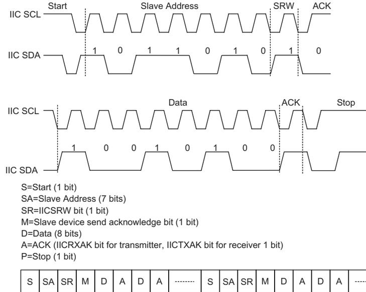
**I<sup>2</sup>C Communication Timing Diagram**
