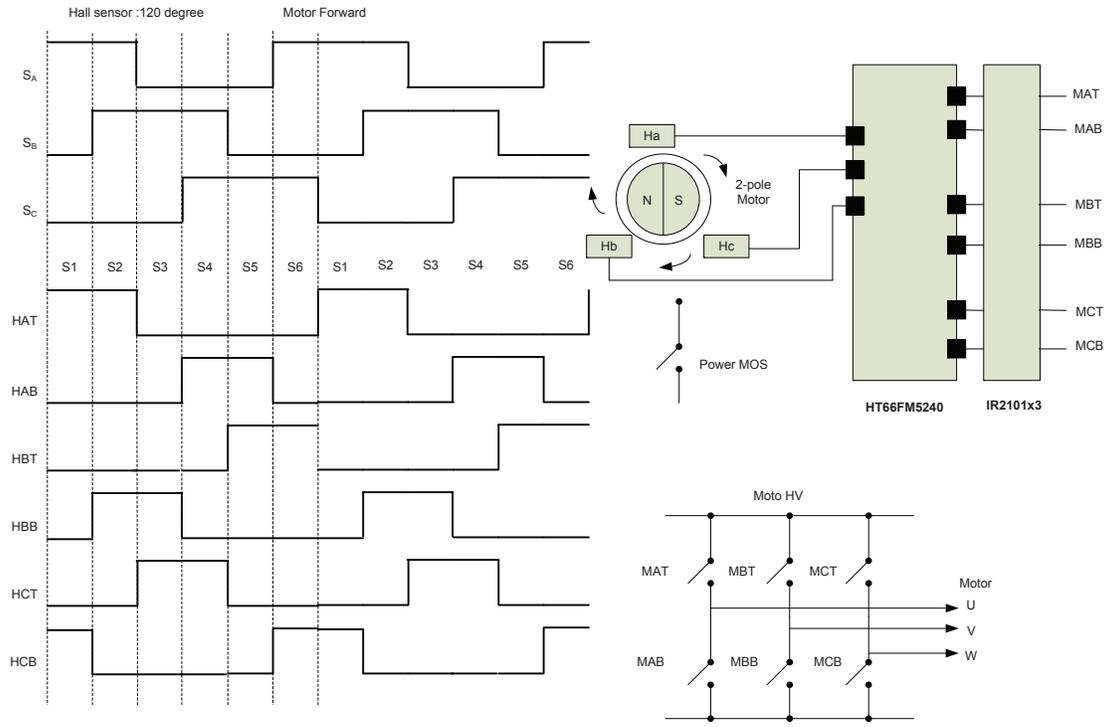
**Motor Drive Signal Timing Diagram – Forward Direction**
